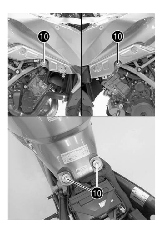
Raise the fuel tank slightly and move it in a backwards direction until it comes out – this may need some careful moving from side to side.
