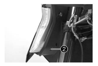
Pull tank spoiler 3 forward and un hook bushing 4 from the inner plastic as shown in picture to release the tank spoiler and then unplug connector 5.
